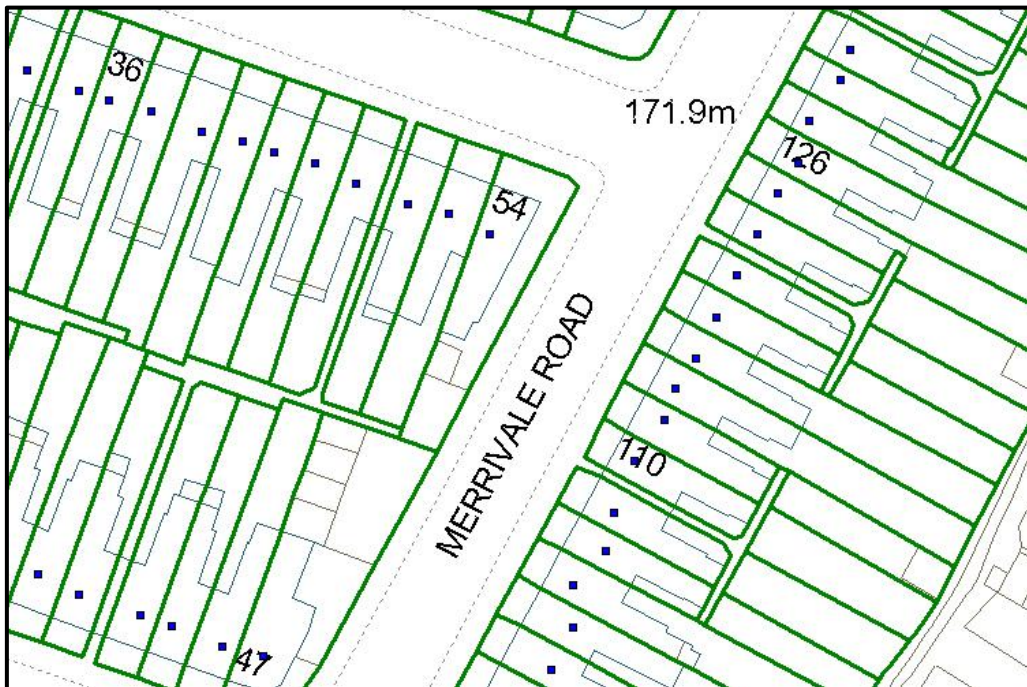
© Crown copyright All rights reserved. Sandwell M.B.C. Licence No 100032119, 2009 Figure 35 - Multi part BLPU Polygon where rear access goes through gardens.
