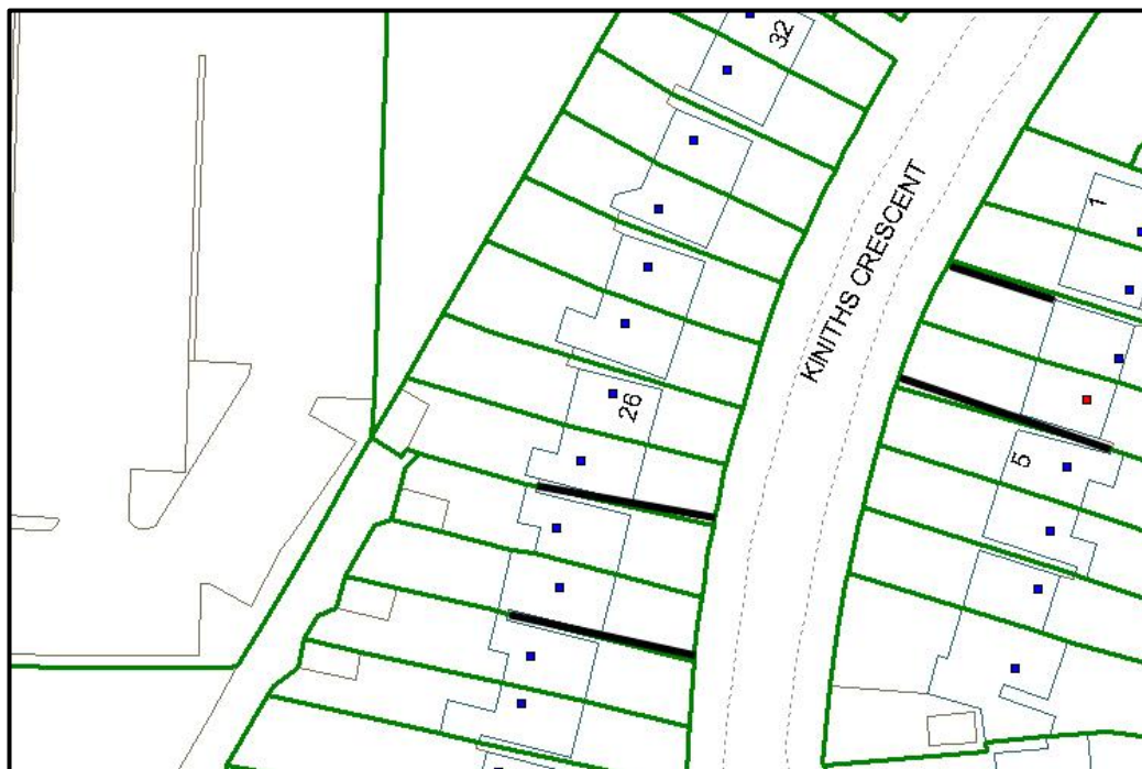
© Crown copyright All rights reserved. Sandwell M.B.C. Licence No 100032119, 2009 Figure 22 - BLPU Polygon extents based on inferred lines if appropriate.
