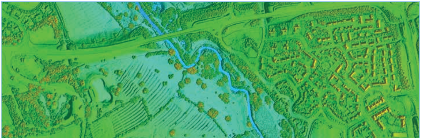
Figure 4 - The image above shows an area as a Digital Surface Model (DSM), which contains the buildings and vegetation. Such objects are removed in the DTM during the data processing stage
