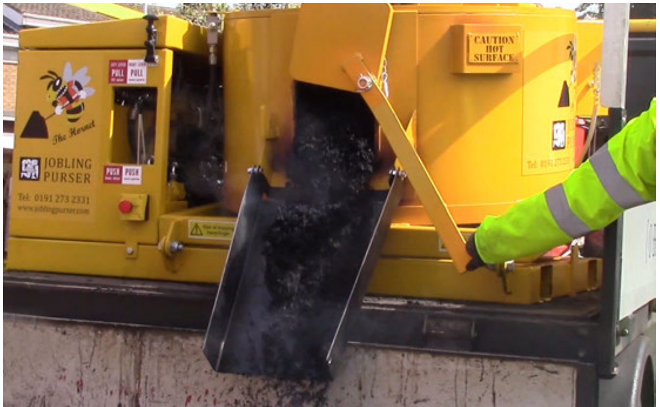
The hot Armaphalt material is ejected from the mixer ready to lay.
